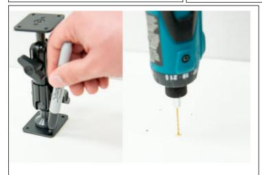
1. Using the pedestal as a template, mark pilot holes for your fasteners.
